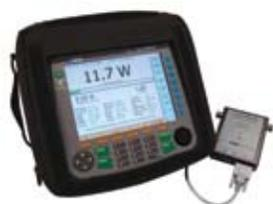
**Power Meter Option:** SignalHawk™ is compatible with Models 5012, 5010B, 5011 and 5011-EF external power sensors. These sensors provide ± 5% (± 0.2 dB) forward average power accuracy. Other measurements include reflected power, VSWR, return loss (dB), peak power, burst average power, crest factor, and CCDF.
