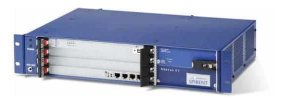
Distributed Abacus 53 protocols include analog FXO and FXS (loop start/ground start), T.30 Fax, V.34 analog data modem, SS7, CAS, MF R1/R1.5/R2, ISDN PRI, GR-303, V5.1/V5.2, SLC-96/TR08 (Mode 1), V.90 Server Data Modem, QSIC (Basic Call Support) on ISDN PRI, BRI over V5.2, RTP/RTCP, Skinny, H.323, SIP, MGCP, H.248.1/ Megaco v1 and v2, NCS, SIP-T, SIGTRAN (M3UA), clear channel signaling, Echo measurements, GRQ - H.235 VoIP gateway message encryption, 3PCC, T.38 Fax over IP.
