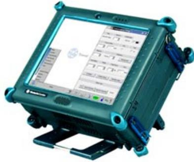
*Victoria Combo Remote Control enables you to control your tester from any where in world. The only requirement is that the Victoria Combo and the PC are connected to TCP/IP networks either physically or using a wireless connection. This means that an engineer can test a network without leaving his desk.*
