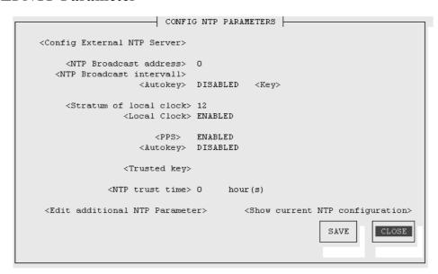
The NTP configuration page is used to set up the additional NTP parameters needed for a more specific configuration of the NTP subsystem.
