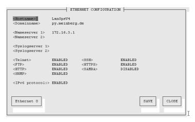
In the network configuration all parameters related to the network interfaces can be changed. In the first section you can change the hostname and domain name. You can also specify two nameservers and two SYSLOG servers. In the nameserver and SYSLOG server fields you may enter an IPv4 or IPv6 address (the SYSLOG servers can be specified as a hostname, too).
