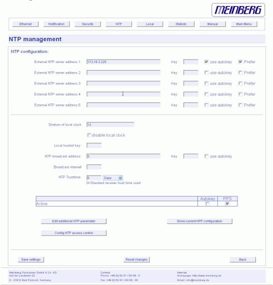
The NTP configuration page is used to set up the additional NTP parameters needed for a more specific configuration of the NTP subsystem.
