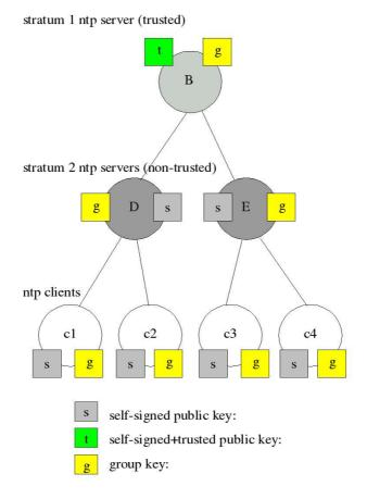
This autokey group is formed by one Stratum-1-server (B), two Stratum-2-servers (D and E) and a number of clients (in the diagram there are 4 clients shown, c1 - c4). B is the trusted host, he holds the group key and a self-signed certificate marked as "trusted".
