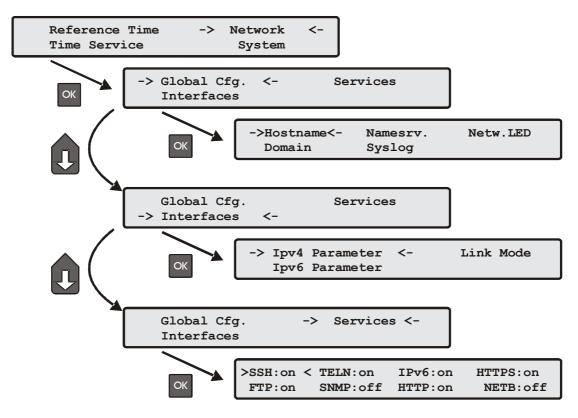
In this submenu the network configuration parameters related to the network interfaces can be changed. The submenus can be selected with the arrow keys and the "OK" button:
