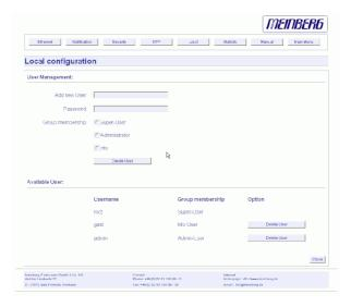
The menu "User Management" allows you to set up different users with a password and the group membership. To change the properties of an user you have to delete the old user and set up a new one. The user "root" cannot be deleted and has always the membership of Super-User. The password of the user "root" can be set on the security page.
