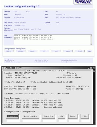
The above screen shots show the web interface and the Command Line Interface setup tool. The CLI setup tool cannot be used by more than one user at a time, the web interface can be used by more than one user in parallel, but the two or more running sessions may influence each other. We explicitly do not recommend the parallel usage of the configuration interfaces.
