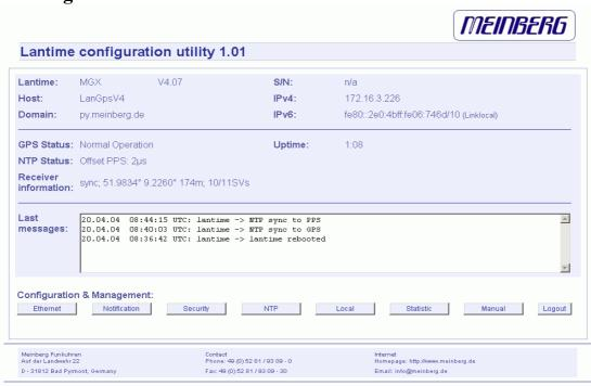
After entering the right password, the main menu page shows up. This page contains an overview of the most important configuration and status parameters for the system.
