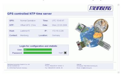
On this start page you see a short status display, which corresponds with the LC display on the front panel of the LANTIME unit. The upper line shows the operation mode of the GPS receiver. As well as "GPS: NORMAL OPERATION" you may also read "GPS: COLD BOOT", "GPS: WARM BOOT" or "GPS: UPDATE ALMANACH". If the connection to the antenna is broken, a "GPS: ANTENNA FAULTY" will appear.
