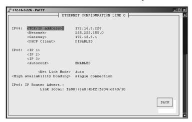
Here, the parameters for the network port can be changed. In the upper section of the page you can enter the IPv4 parameters, the lower part gives you access to the IPv6 parameters of the interface.
