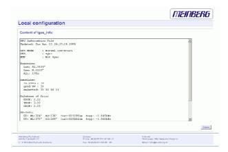
The accuracy of the calculated receiver position and time deviation is dependent on the constellation of the four selected satellites. Using the position of the receiver and the satellites, a number of values can be calculated, which allow a rating of the selected constellation. These values are called "Dilutions of Precision (DOP)".
